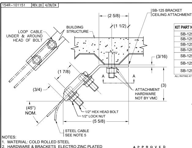
MAX. TENSION ALLOWABLE(LBS. KIT KIT PART NUMBER COLOR CODE **TYPE** SLOT/HOLE SB-125-01 CLEAR ZINC COATED 9/16" SB-125-02 YELLOW ZINC COATED SLOT/HOLE 11/16" SB-125-03 CLEAR ZINC COATED HOLE 9/16" SB-125-04 YELLOW ZINC COATED 1100 HOLE 11/16" 9/16" CLEAR ZINC COATED HOLE SB-125-05 11/16' YELLOW ZINC COATED SLOT HOLE 11/16" YELLOW ZINC COATED SB-125-06 SLOT 9/16' **CLEAR ZINC COATED** HOLE 11/16 YELLOW ZINC COATED SB-125-07 9/16' CLEAR ZINC COATED HOLE
